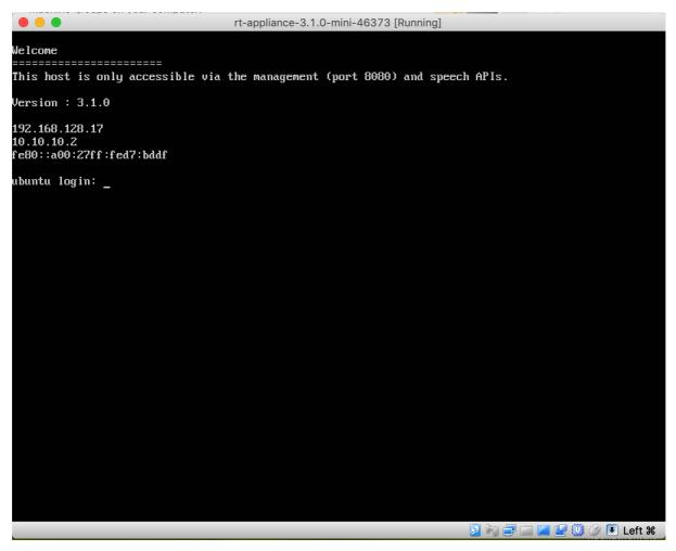
The screen shot above shows the 10.10.10.2 IP address as the fallback address. The other address shown was allocated by DHCP and should be used for all communication.
